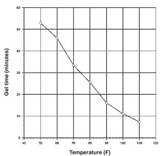
This graph shows gel time as a function of temperature. With the curve being basically linear, a good rule of thumb is 30 minutes (approx.) at room temp. ( $72^{\circ}$  F) and varies about 1 minute per degree temperature change.
