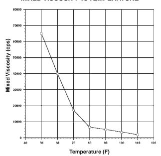
This graph shows viscosity is relatively constant above 80° F, but changes rather dramatically between 70° F and 50° F. This can be very noticeable when pouring on concrete which may be 10-20° F cooler than the ambient air temperature.
